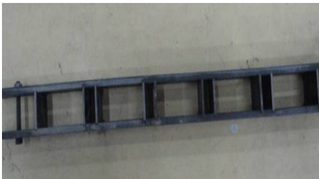
Fig. 1: Steel mould for casting fly-ash concrete bricks
