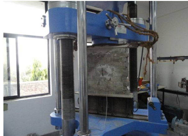
Fig. 4: Loading arrangement for testing under cyclic compressive loading
